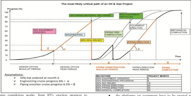
Piping completion works, from 85% erection progress to mechanical completion, i.e., all pipe-work installed, supported, tested, insulated, is best modeled as a constant, typically 6 months on a large job.
